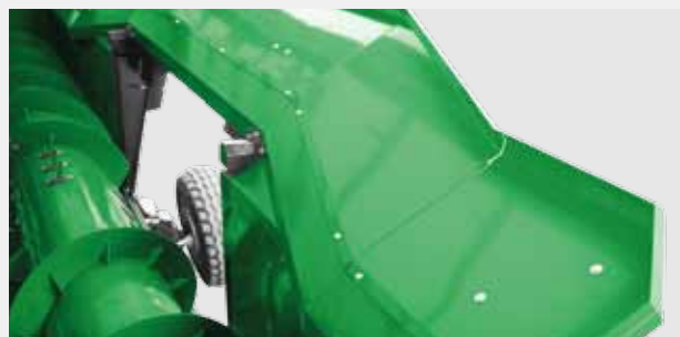
SPLASHGUARD to prevent grain losses around the feeder house area
