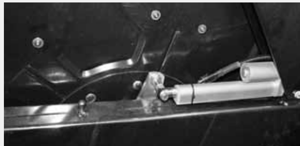
ELECTRIC REEL TINE ADJUSTMENT flat angle for rape – steep angle for flat crop
