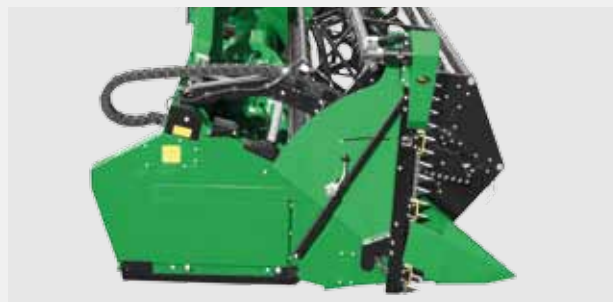
INTEGRATED ELECTRIC OR HYDRAULIC SIDE KNIVES can also be used in combination with crop dividers (for instance rye)
