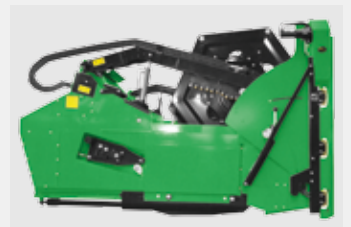
CUTTING KNIFE COMPLETELY EXTENDED and side knives folded-up
