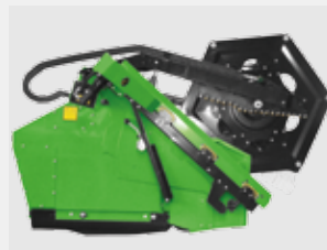
CUTTING KNIFE COMPLETELY RETRACTED and side knives folded
