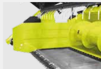
CUTTING KNIFE COMPLETELY EXTENDED Distance to intake auger 1070 mm
