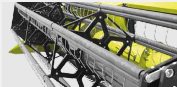
WRAP PROTECTION FOR THE REEL prevents the wrapping of weeds (for instance camomile) around the reel tine tubes
