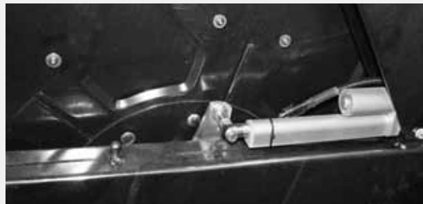
ELECTRIC REEL TINE ADJUSTMENT flat angle for rape – steep angle for flat crop
