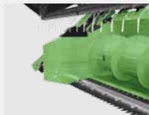
CUTTING KNIFE COMPLETELY RETRACTED Distance to intake auger 370 mm
