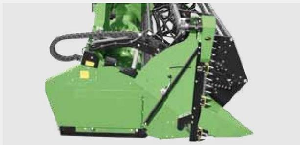
**LAME COLZA INTEGRATE A COMANDO ELETTRICO O IDRAULICO**
