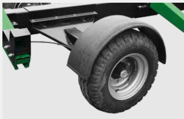
40 KM/H DESIGN (MUDGUARDS, FOUR-WHEEL BRAKE ETC.)
