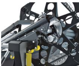
integrated hydraulic reel drive in the main tube , smooth crop floor
