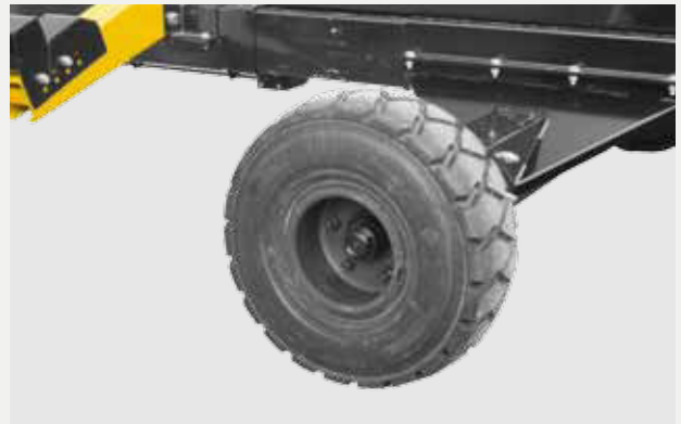
LOW TYRES FOR SWIFT Absolutely necessary for combines with limited lifting
