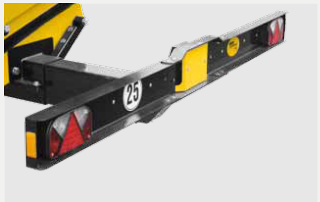
HIGHER POSITIONED LIGHT BAR To avoid damages at steep field entrances
