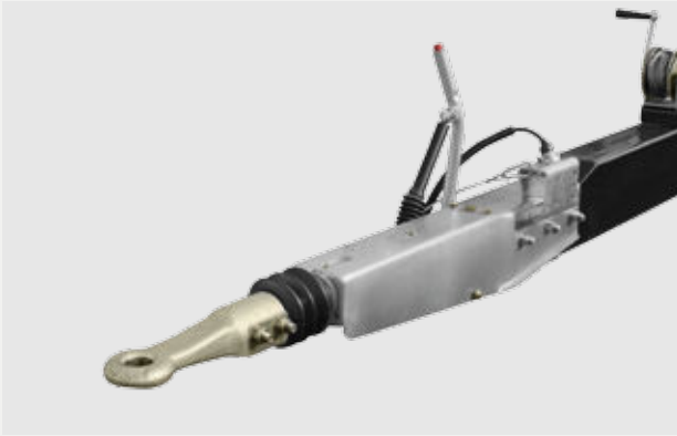
OVERRUNNING- AND PARKING BRAKE FOR SWIFT AND TANDEM For better driving comfort
