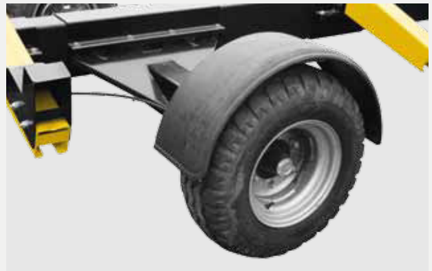
40 KM/H DESIGN (MUDGUARDS, FOUR-WHEEL BRAKE ETC.) Available for all BISO header trailers
