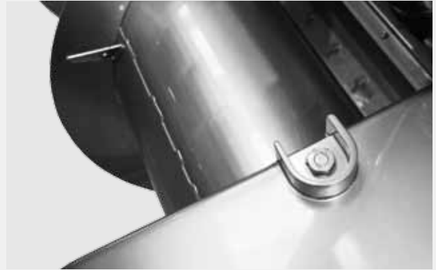
EASY AUGER HEIGHT ADJUSTMENT for thick rape stalks
